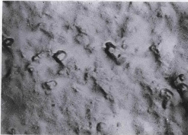
Figure 9 ELECTRON MICROGRAPHS OF HIGH DENSITY MgO
