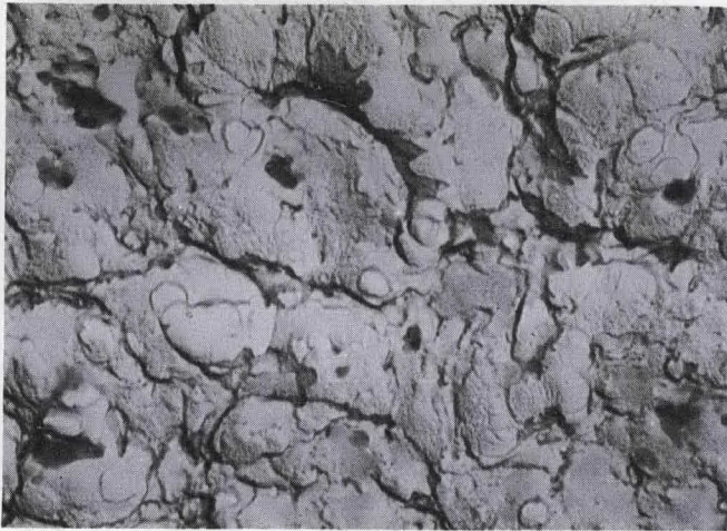
Figure 8 ELECTRON MICROGRAPHS OF HIGH DENSITY MgO
