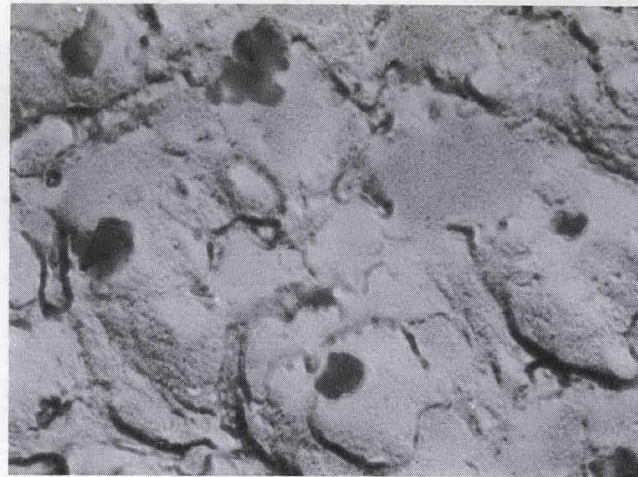
Figure 8 ELECTRON MICROGRAPHS OF HIGH DENSITY MgO
